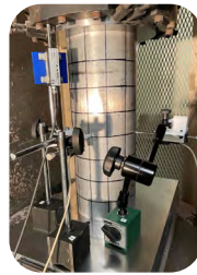
Fig. 5. Stub column test set-up
